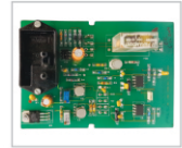
Pressure Transducer PCB
